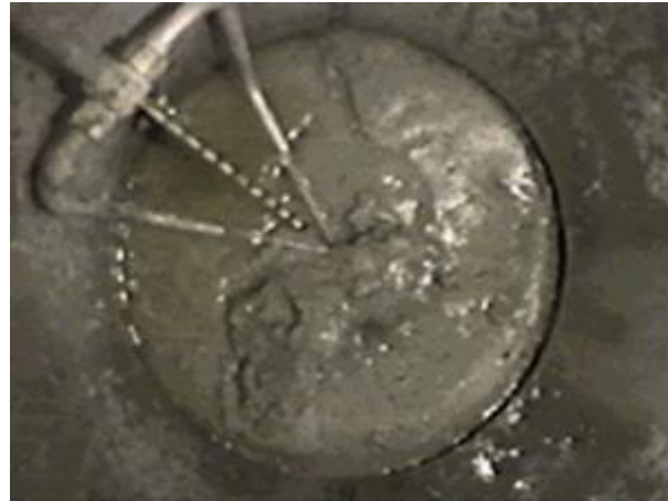
View of clean shaft bottom through Mini-SID camera with 1/4 inch of sediment
